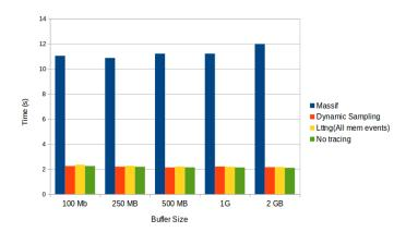
Fig. 5. Tracing impact on execution time
