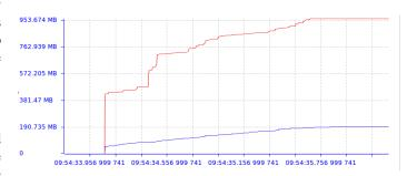
Fig. 7. Firefox memory usage at startup using LTTng
